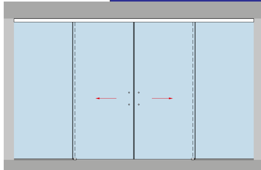
Double leaf sliding + 2x Fixed panes to inside of reveal
